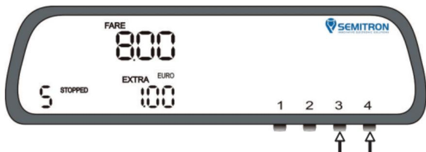
During “STOPPED” mode hold button 3 and press button 4 to delete any added extra.
