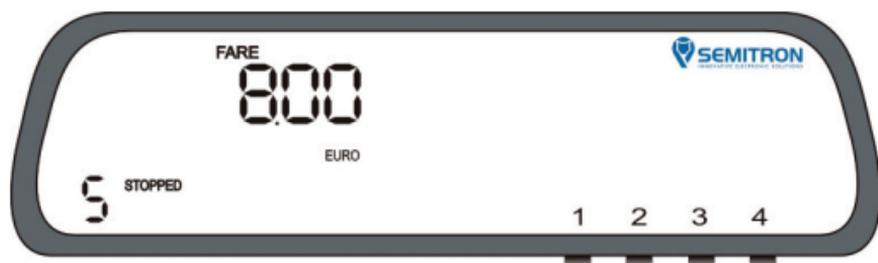
During this operational mode the taximeter displays the charged amount (fare + extra). Signs “FARE”, “STOPPED”, “EURO” and letter ‘S’ are displayed. Press button 1 for cash or button 2 for credit in order to end current hire.
