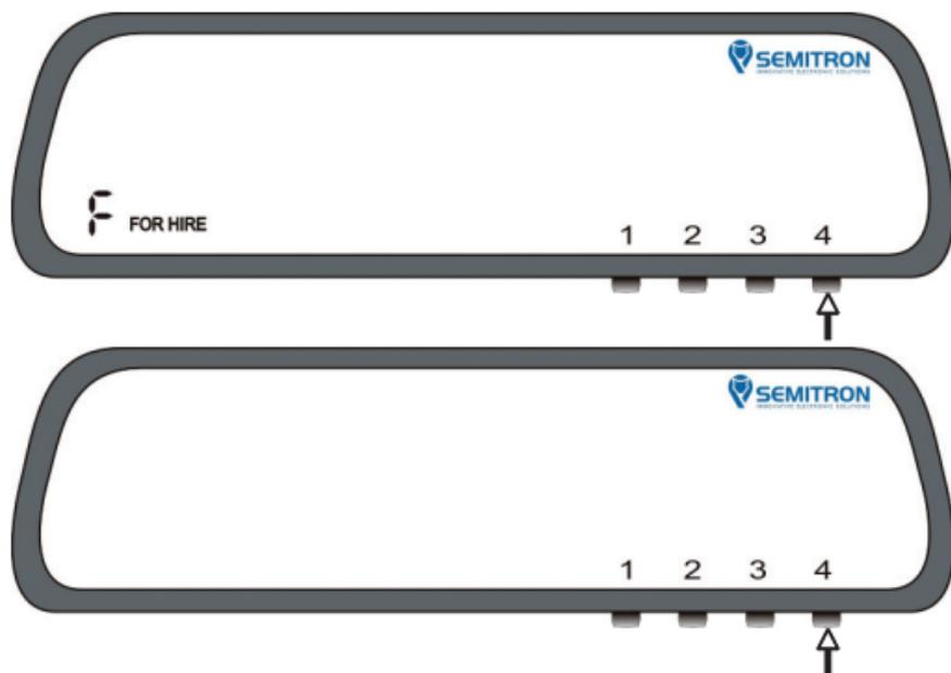
During “FOR HIRE” or “CLOSED” mode press button 4 to enter in auxiliary menu.
