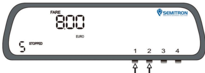
During “STOPPED” mode press button 1 to charge cash or press and hold button 2 for 3 seconds to charge credit. The taximeter will print a receipt (if it is programmed).
