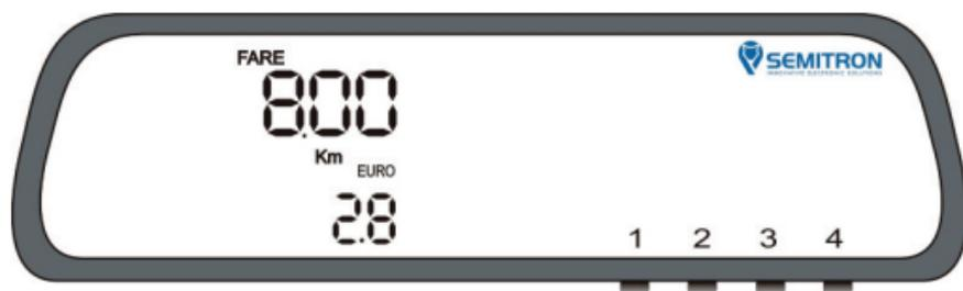
Fare and Extra (and km after 3 seconds), of the last hire of the current shift will be displayed. If the current shift has no hire yet, then nothing will be displayed.
