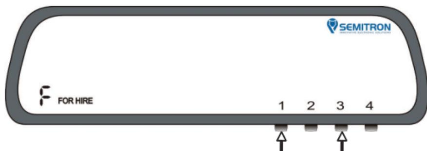
During “FOR HIRE” mode hold button 3 and press button 1 to change the brightness.
