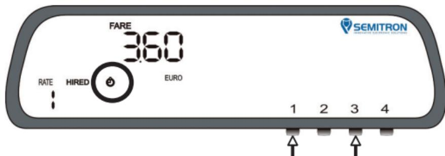
During “HIRED” mode hold button 3 and press button 1 to enable or disable the time - charge. If the time – charge is enabled the “Clock” sign will be on.
