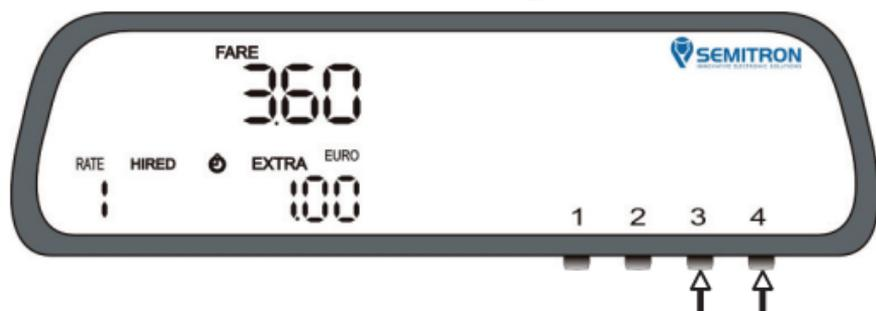
During “HIRED” mode hold button 3 and press button 4 to delete any added extra.
