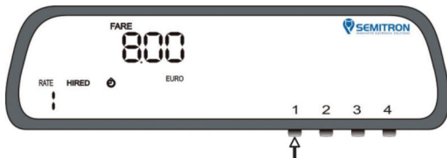
During “HIRED” mode press button 1 to go to “STOPPED” mode.
