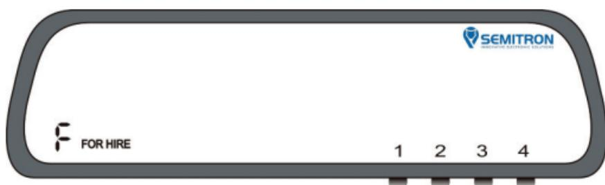
During this operational mode the taximeter does not calculate any charges. Information about distance travelled without passenger is registered. Letter ‘F’ and sign “FOR HIRE” are displayed. Press button 2 to enter in “HIRED” mode.
