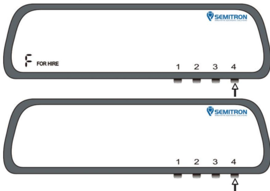
During “FOR HIRE” or “CLOSED” mode you can adjust time up to 2min/week by using calend option from the auxiliary menu. Press button “4” 7 times consecutively to find the Calend menu.
